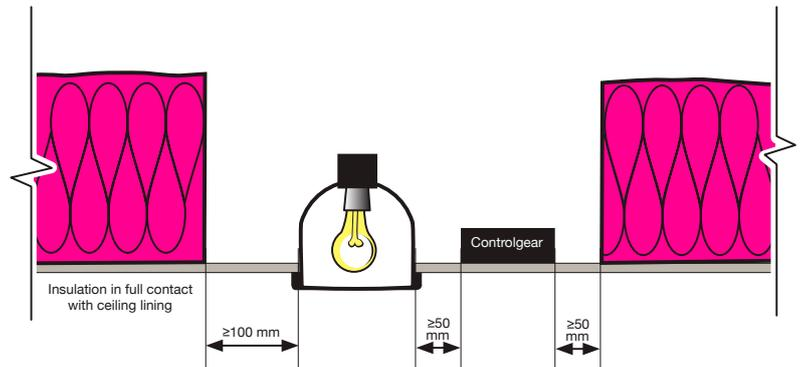
Unmarked luminaire and controlgear not placed on top of Pink® Batts® ceiling products.
