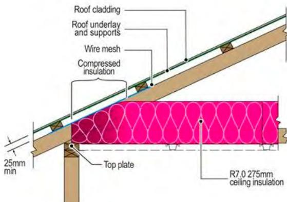
**Note:** Pink® Batts® ceiling insulation can be installed from below when the ceiling is to be lined or replaced
